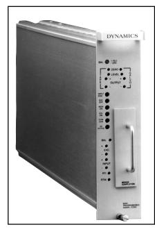
gauges, RTDs and potentiometers. Each conditioner is fully guarded and isolated as required to maintain signal integrity. System hardware consists of three major components: Model 8000 Signal Conditioner/Amplifiers, a Master Rack and a Slave Rack.
