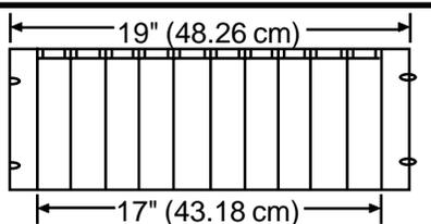
Dynamics cabinets are constructed of 20-gauge cold-rolled steel. Multi-channel cabinets meet all standard EIA mounting requirements.
